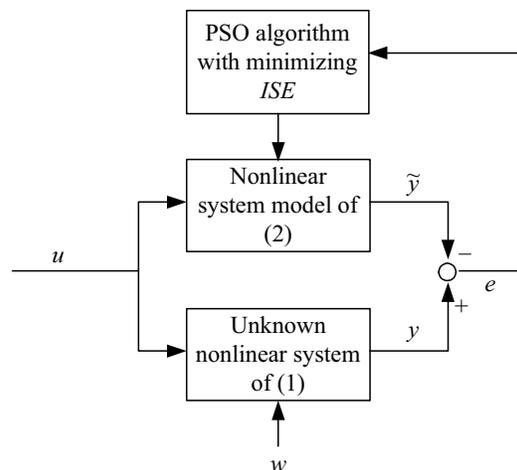
Figure 1. PSO algorithm estimation of nonlinear systems with measurement noise.
