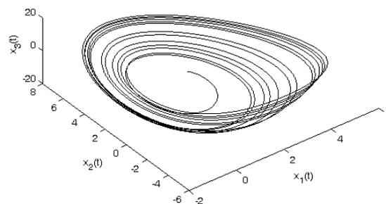
Figure 2. Three-dimensional phase portrait of states  $x_1$ ,  $x_2$ , and  $x_3$  for the unforced Genesio-Tesi chaotic system.
