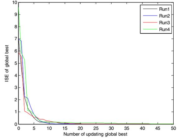
Figure 4. Convergence curves of objective function  $ISE$  under  $w \in [-0.01, 0.01]$ .
