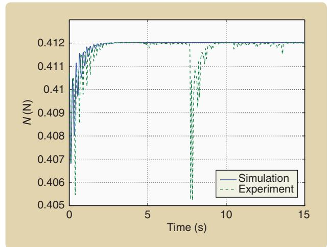
**FIGURE 9** Simulation and experimental results for the response of the normal force  $N$  in Newtons. The initial conditions are  $\theta_1(0) = -0.08$  rad,  $\dot{\theta}_1(0) = 0$  rad/s,  $\theta_2(0) = 0.08$  rad, and  $\dot{\theta}_2(0) = 0$  rad/s. Since  $N$  remains positive for all time, the ball does not leave the wheel.
