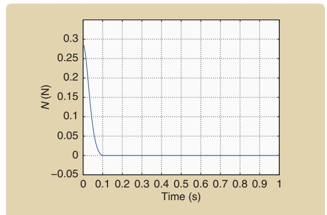
**FIGURE 10** Simulation result of the response of  $N$ . To verify that a sufficiently large initial angular position of the ball can result in the ball leaving the wheel, the initial condition is chosen to be  $[\theta_1(0) \ \dot{\theta}_1(0) \ \theta_2(0) \ \dot{\theta}_2(0)] = [0.8 \text{ rad} \ 0 \ 0 \ 0]$ . Note that  $N = 0$  at time 0.1 s, at which time the simulated ball separates from the wheel and  $N$  remains zero.
