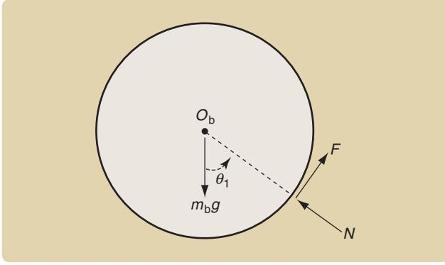
**FIGURE 5** Free-body diagram of the ball.  $N$  denotes the normal reaction force due to the wheel, while  $F$  denotes the frictional force. The external force  $m_b g \cos \theta_1 - N$  provides the centripetal acceleration necessary to keep the ball rolling on the periphery of the wheel.
