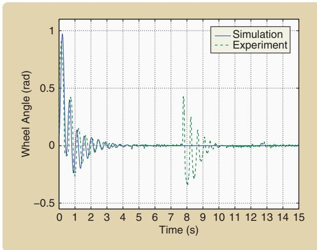
**FIGURE 7** A comparison of simulation and experimental results of the angular position response of the wheel. The initial conditions are  $\theta_1(0) = -0.08$  rad,  $\dot{\theta}_1(0) = 0$  rad/s,  $\theta_2(0) = 0.08$  rad, and  $\dot{\theta}_2(0) = 0$  rad/s. The motor rotates the wheel to bring the ball to the equilibrium. The oscillation at time 7.6 s is the response to the impulsive disturbance induced in the experiment by tapping the ball.
