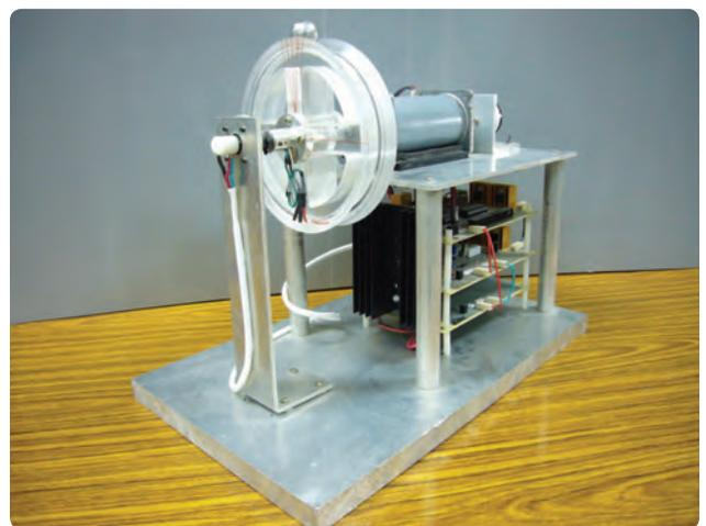
**FIGURE 1** Experimental setup of the ball and wheel system. The wheel is controlled by a dc motor. The objective is to stabilize the ball over the periphery of the wheel at its unstable equilibrium. The system is nonlinear and underactuated.
