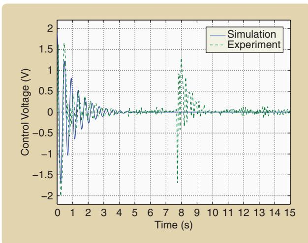
**FIGURE 8** A comparison of simulation and experimental results of the control voltage. The operating range of the control voltage is  $\pm 20$  V, which is constrained by the motor driver. The control voltages are not saturated in either the simulation or the experiment.
